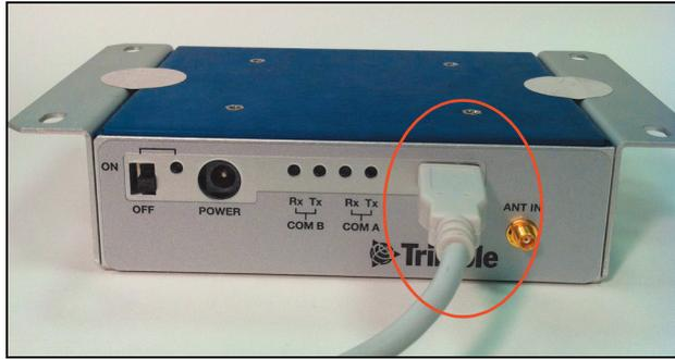
2. Connect the other end of the USB cable to your computer. The USB cable now supplies power to the unit.
